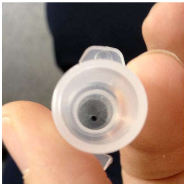
Figure 1: Transparent plastic membrane at the opening of the ETT connector with an orifice with a diameter of 2 mm
