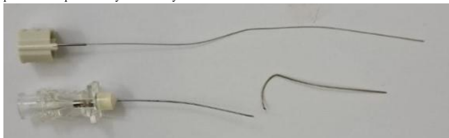
Figure 1: 27G Quincke spinal needle with its broken fragment that was buried in the spine and removed surgically.
