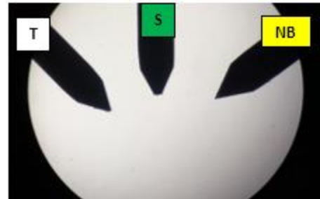
Figure 1: Satisfactory blunting following 'scraping method'. T-tapped, S-scraped, NB- non-blunted (Optical microscopic view 40x)
