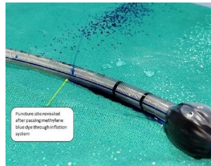
Figure 1: ETT showing leak of methylene blue dye from breakage site
