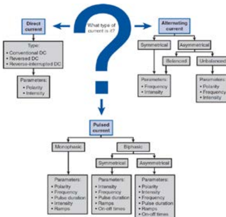
Figure 1: Classification of electrical current 13
